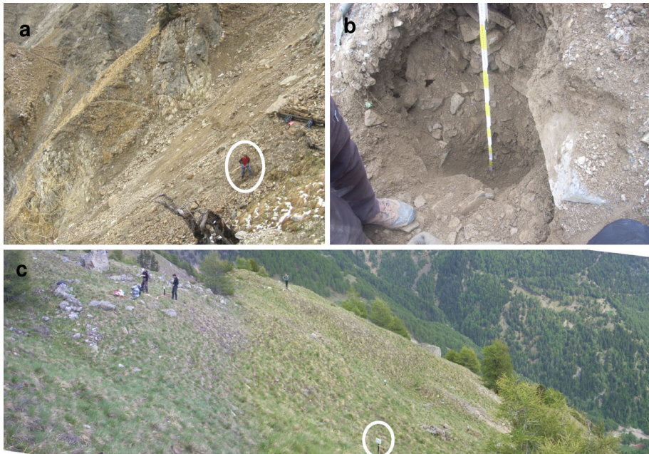
Fig. 5 Images of the sites equipped to monitor hillslope hydrology: a the most active channel head at S1 (a person is circled for scale) and b the hole where the pore pressure transducer was installed; c a panoramic view of site S2 where the soil moisture probes (one datalogger is marked) and piezometers are installed
