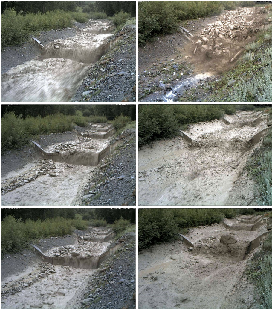
Fig. 10 Frames from the video camera at station D2. Left column : the three surges of August 2011 event (surge 1 above, surge 2 in the middle and surge 3 below, as in Table 2); right column : three snapshots of the July 2013 debris flow, with the initial front above, the central part of the event in the middle, and a late surge transporting a large boulder below (the one marked in Fig. 9)
