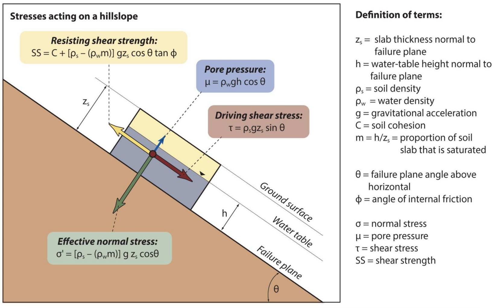
The **infinite-slope model** is often used to analyze the stability of slopes to shallow, planar landslides. The model is a balance between the **shear strength** of the slope materials and the **shear stress** provided by gravity, due to the downslope-oriented component of the mass of the soil. It considers the **pore pressure** effect on the stress balance as well as the effect of slope.
